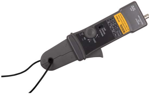
Figure 2 Connection between the Test Clamp and Conductor
